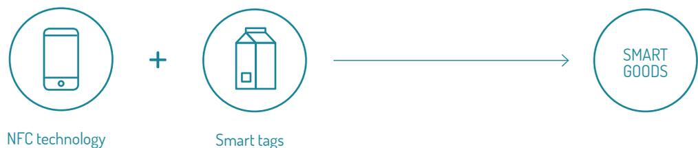
TagItSmart! uses functional inks and printable electronics to create context-sensitive smart tags. The smart tags change dynamically according to the environment and exposure (e.g. temperature and oxygen exposure). The universally available smart phone can be used to capture and transmit information from these
